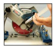
Turn the saw over and drain all the oil for at least 2 minutes (oil has to be warm to drain).
