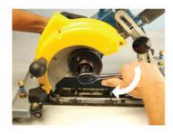
Remove Motor Mount Screws
