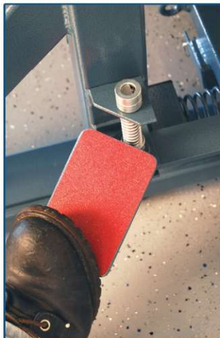
Vertical lock with foot pedal release
