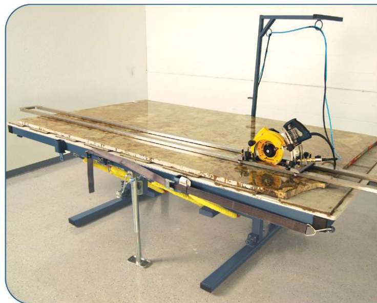
Power and water boom keeps your cords off the table.
