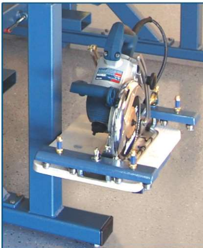
Saw stand for out-of-the-way storage
