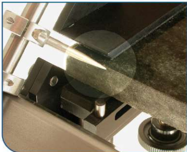
3. Calibrate Tracks to blade cut line with Calibration Indicators.
