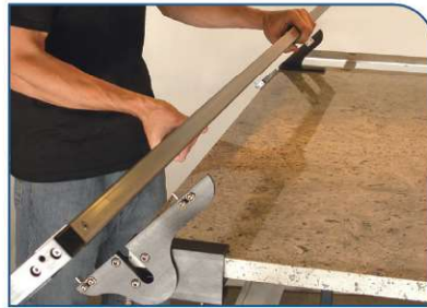
2. Place the Track on the fixtures.
