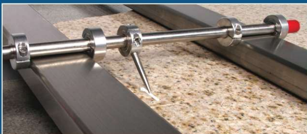
2. Place Tracks on cut line
