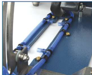
Four water tips for equal flow to both sides of the blade. No adjustment needed.
