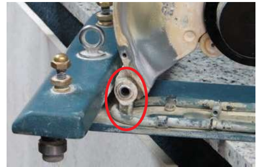
There are 2 Heim Joints, one on each side of the blade guard.
