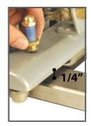
NOTE: to install new Glide Pins, first remove the old pins counterclockwise and clean the threaded holes. Replace with new Glide Pins and turn them clockwise, 3/16" to 1/4" past the bottom of the saw.
