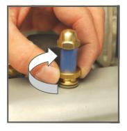
**5.** When the blade is square on the track and no rocking occurs, tighten the brass lock nuts clockwise. Be careful not to turn the Glide Pins while tighteing.
