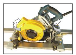
**B)** For a gap a the top of the square, adjust the two motor-side Glide Pins evenly until until no light shows through between the blade and square.
